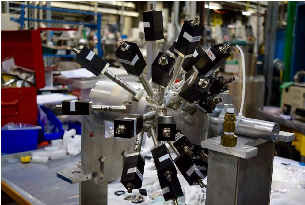
Figure 3.24: The new scattering chamber SONIK which can be set-up around the windowless gas target at DRAGON. (Picture: 2018 TRIUMF Photowalk; Sarah Johnson)
