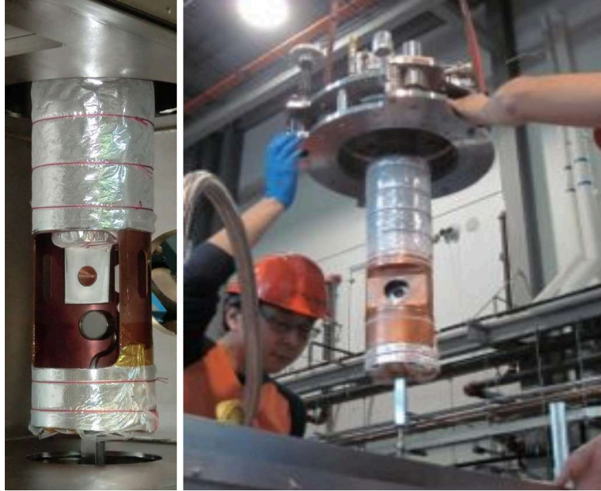
Figure 3.16: Views of the solid hydrogen or deuterium target assembly of the IRIS detector at TRIUMF-ISAC-II.
