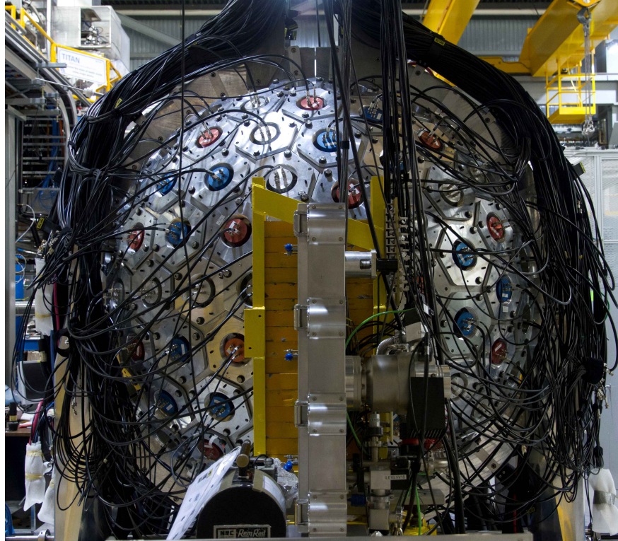
Figure 3.15: A photograph of the 70-element DESCANT neutron detector array coupled with the GRIFFIN spectrometer at ISAC-I.
