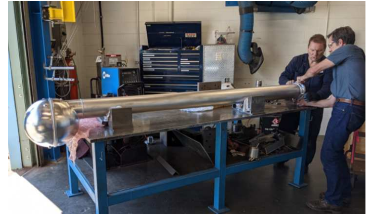
UCN production volume prepared at TRIUMF, now being prepared for final welding, Nov. 2022
