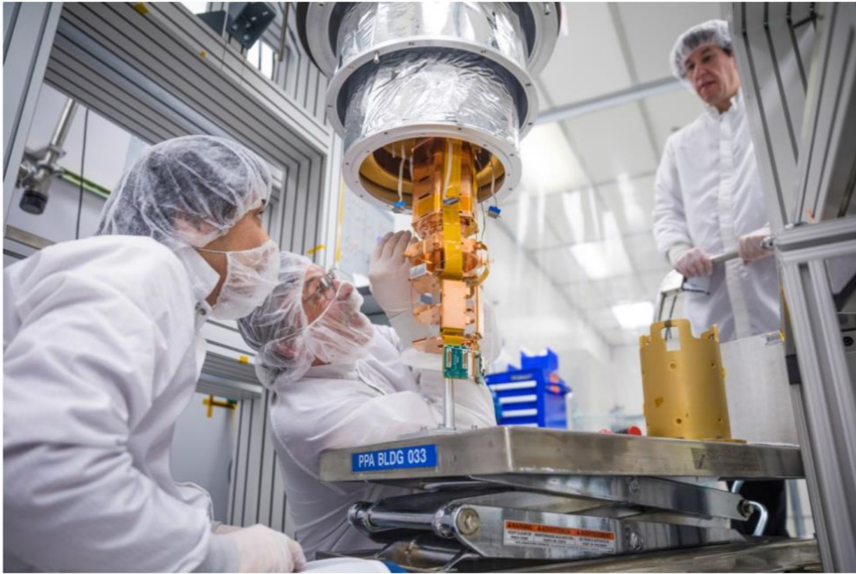
The SLAC team inspects an installed tower at the bottom of the dilution refrigerator used for tower testing. | Image: Christopher Smith/SLAC National Accelerator Laboratory
